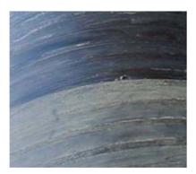
Step 4: Visually inspect the joint to ensure that male and female threads are engaged.
